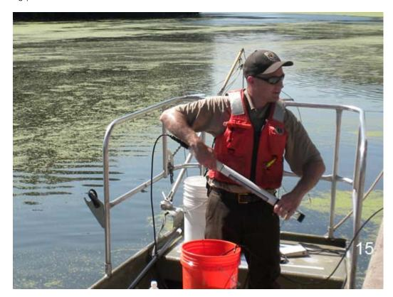
Following the demonstration, Goehle used some water sampling equipment - a plankton net (13) and hydrolab (15) to, respectively, collect plankton and larval fish [examined by teachers in a plastic container, (14)] and run some standard tests (pH, turbidity, water temperature, and dissolved oxygen).
